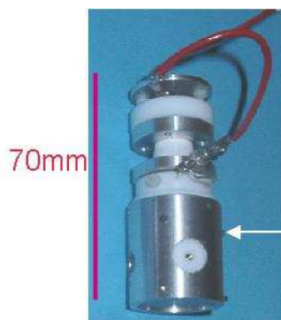
Figure 4.3 Prototype, ruggedized ion trap mass spectrometer
