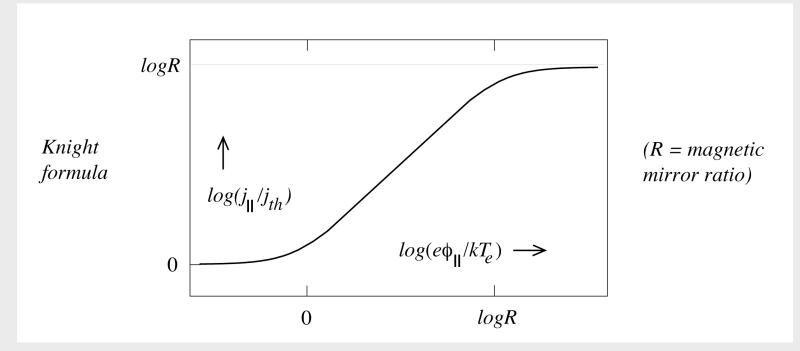
Upward  $j_{||}$  requires a downward electron flux, which requires  $\phi_{||}$  to overcome the magnetic mirror force.
