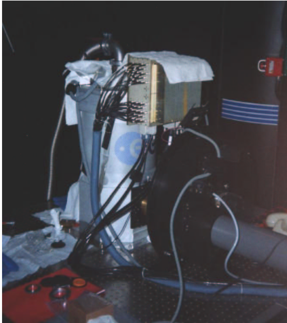
Figure 2.5: The S-Cam 2 instrument at the Nasmyth focus of the William Herschel Telescope, La Palma. The pipe in the lower right encloses the telescope light feed and leads to the instrument filter wheel. Above this are the individual pixel electronics. The cryostat is partially visible behind the filter wheel. (Photograph by the author).
