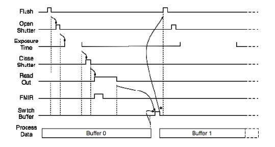
Note: The FMIR is moved while the read-out is active (only for scanning raster)
