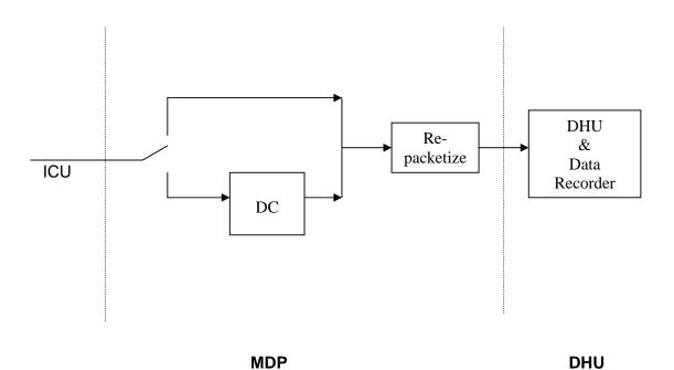
The spacecraft data handling system consists of two parts, the Mission Data Processor (MDP) and the Data Handling Unit (DHU).
