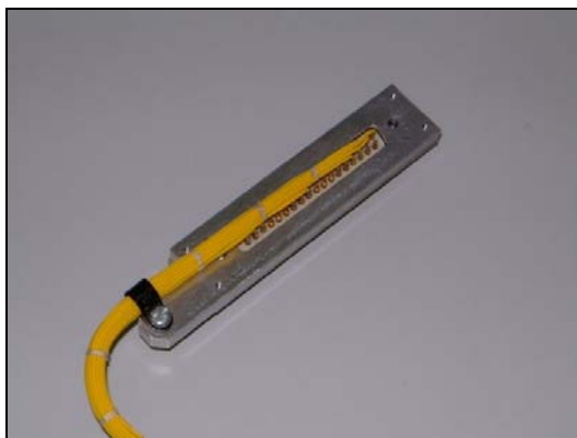
Fig. 5 Mechanism connector and P clip.
