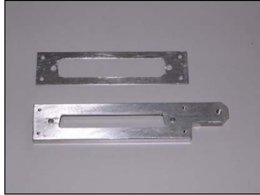
Fig. 2 Connector mounting bracket.
