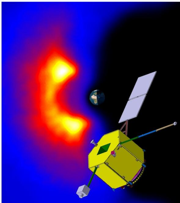
AXIOM spacecraft concept drawing with simulated X-ray emission from the Earth's dayside magnetosphere (for more on the X-ray simulations see <http://www.star.le.ac.uk/~jac48/pxsims/>)
