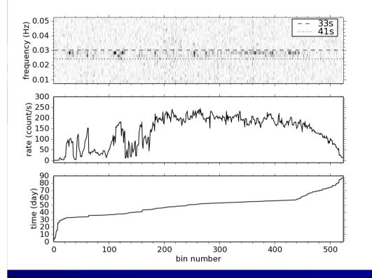
*P* ~36s modulation apparent during SSS phase prior to linear decline
