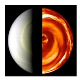
Venus Express carries onboard an instrument that peers below the thick Venusian clouds using a 'window' in the infra-red portion of the spectrum. The image to the left is a composite of the day half (left) and night half of the planet (right). The day half shows sunlight reflected from the tops of clouds, whereas the night portion is seen by peering below the cloud using the infra-red window.
