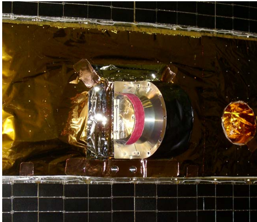
Figure 8. Photograph of TC-2 PEACE Sensor head showing arrangement of electrostatic conductive materials; spacecraft and PEACE thermal blankets and also solar cells above and below the experiment platform. Note the larger collimator of a LEEA sensor vs. the TC-1 HEEA sensor.
