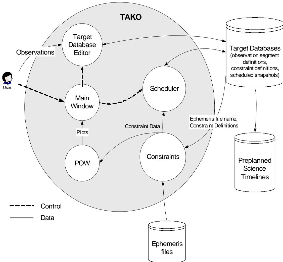
Figure 1.2-1 TAKO Data and Control Flow Diagram
