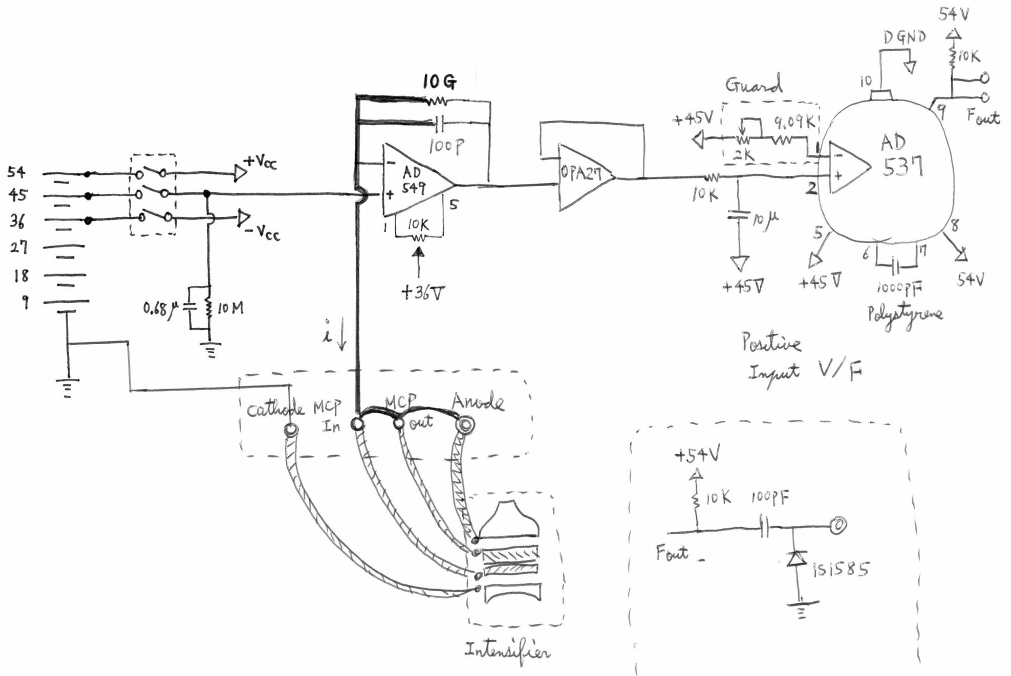
Fig. 4 Photocathode current amplifier
