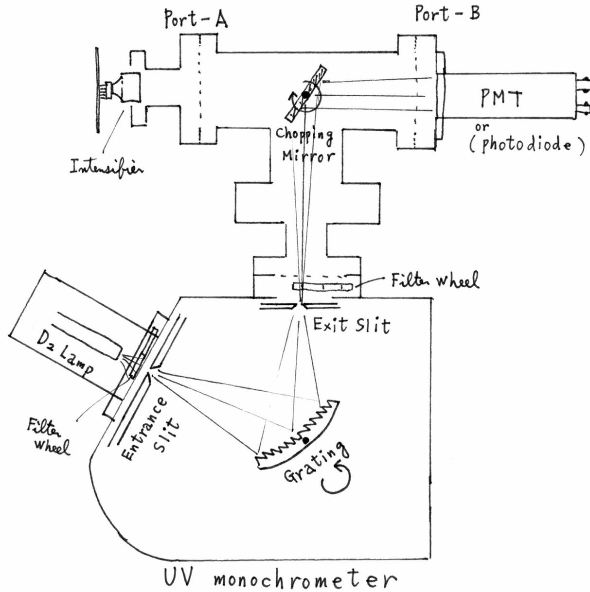
**Fig. 2** Optics configuration of Q.E. measurement
