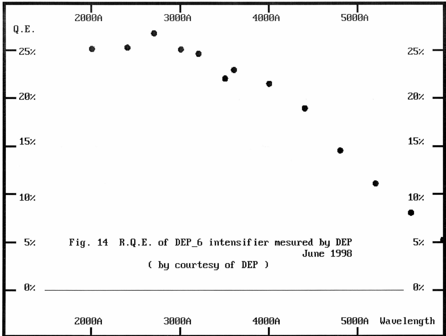
Fig. 14 R.Q.E. of DEP\_6 intensifier mesured by DEP
