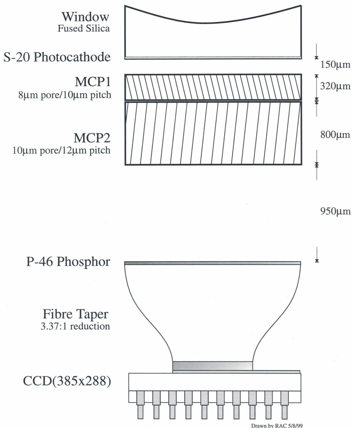
Schematic Structure of Detector Head
