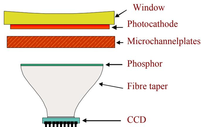
*Figure 1: Schematic of the MIC detector*
