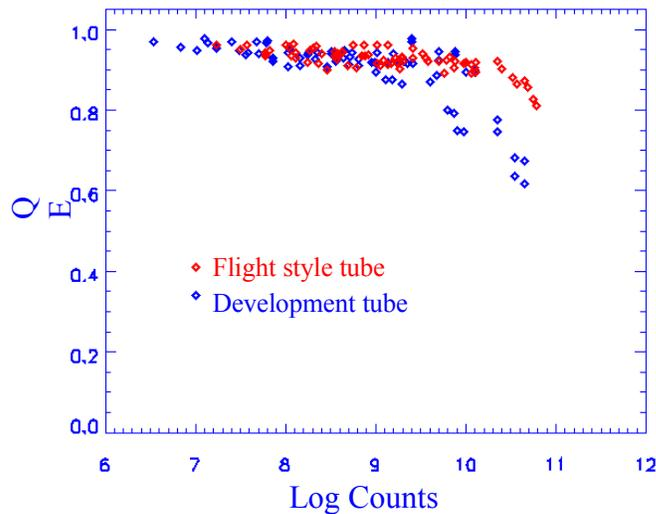
Figure 2: Quantification of cumulative damage to the MIC detector
