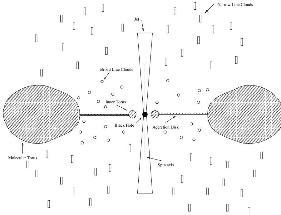
Figure 1.1: A schematic diagram of an active galactic nucleus (Not to scale). The central black hole is surrounded by an accretion disk, which may have an inner torus. The accretion disk is inside the molecular torus. The broad and narrow line clouds are somewhere above the accretion disk plane. Narrow line clouds are further from the black hole than the broad line clouds. There are a pair of jets launched from some region close to the central black hole.
