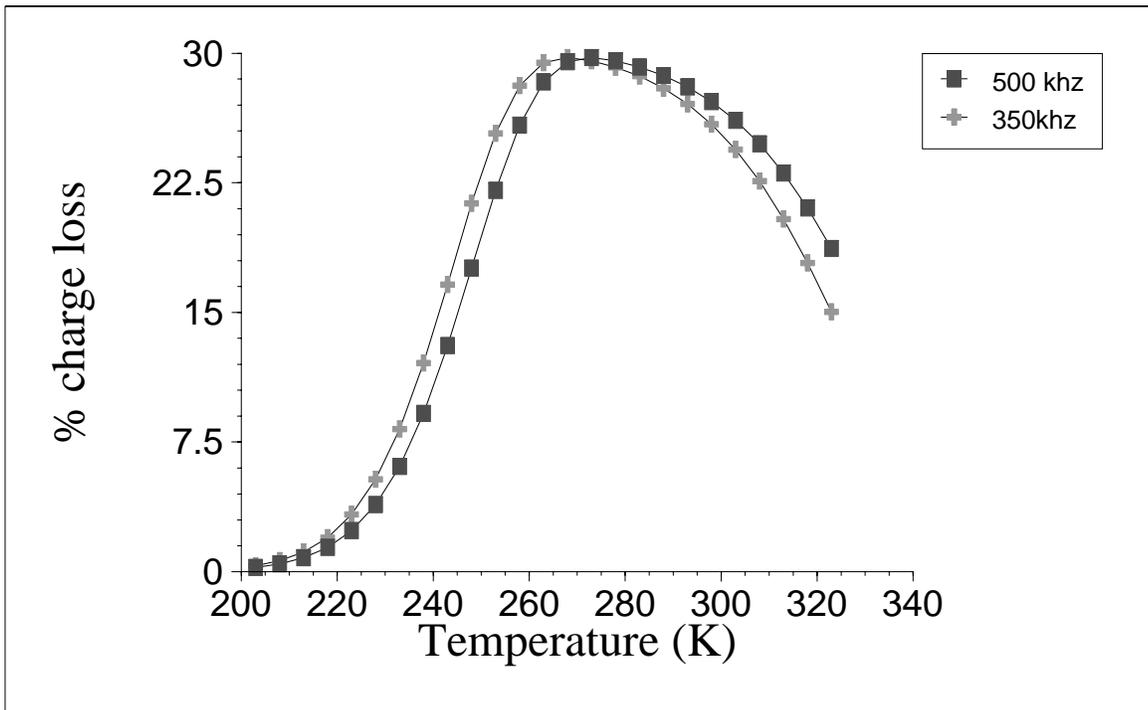
CTI loss for 1000 electrons, for 2 clocking rates
