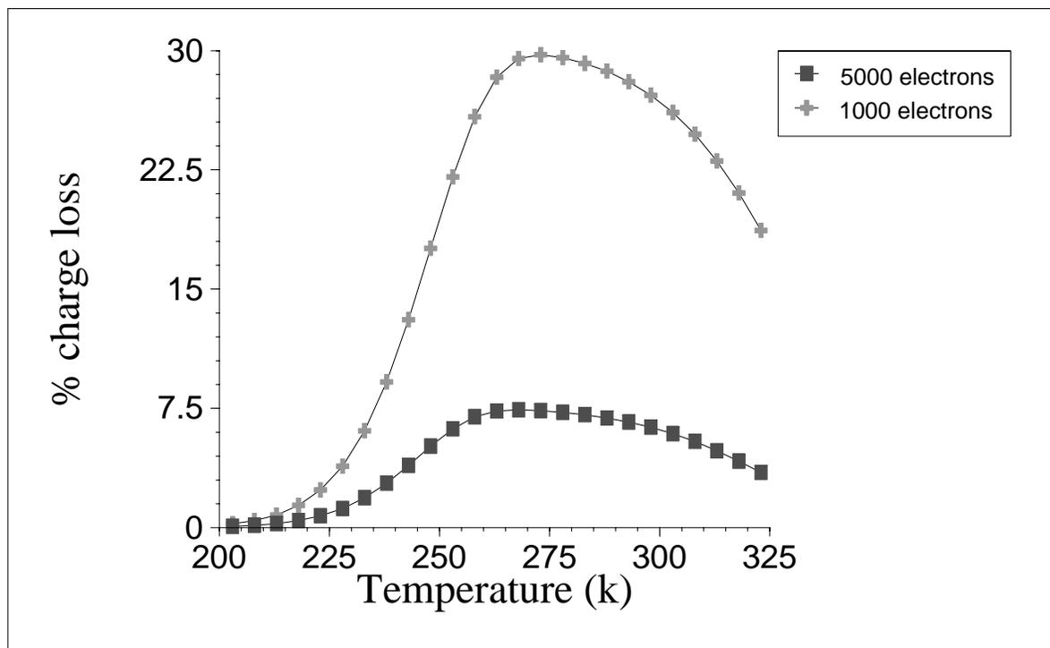
%charge loss for 1000 and 5000 electrons, for 500kHz clocking
