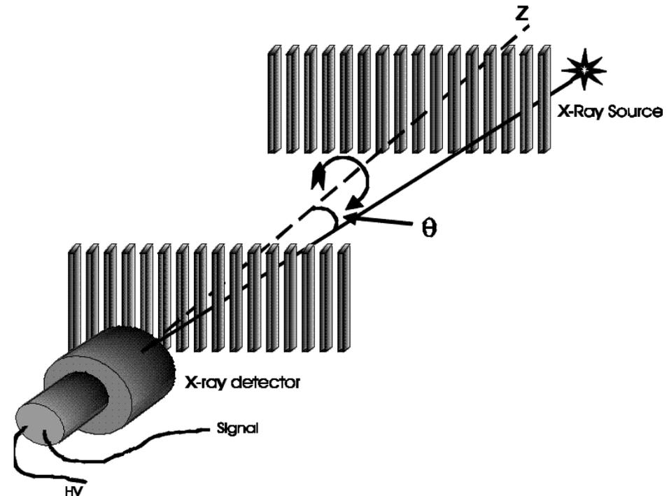
Incoming X-ray flux is modulated by a pair of grids – modulated lightcurves are used later to recover spatial information
