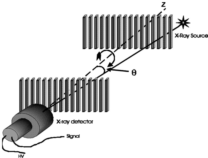
RHESSI detectors look at the source through a pair of grids called **Rotating Modulating Collimator (RMC)**
