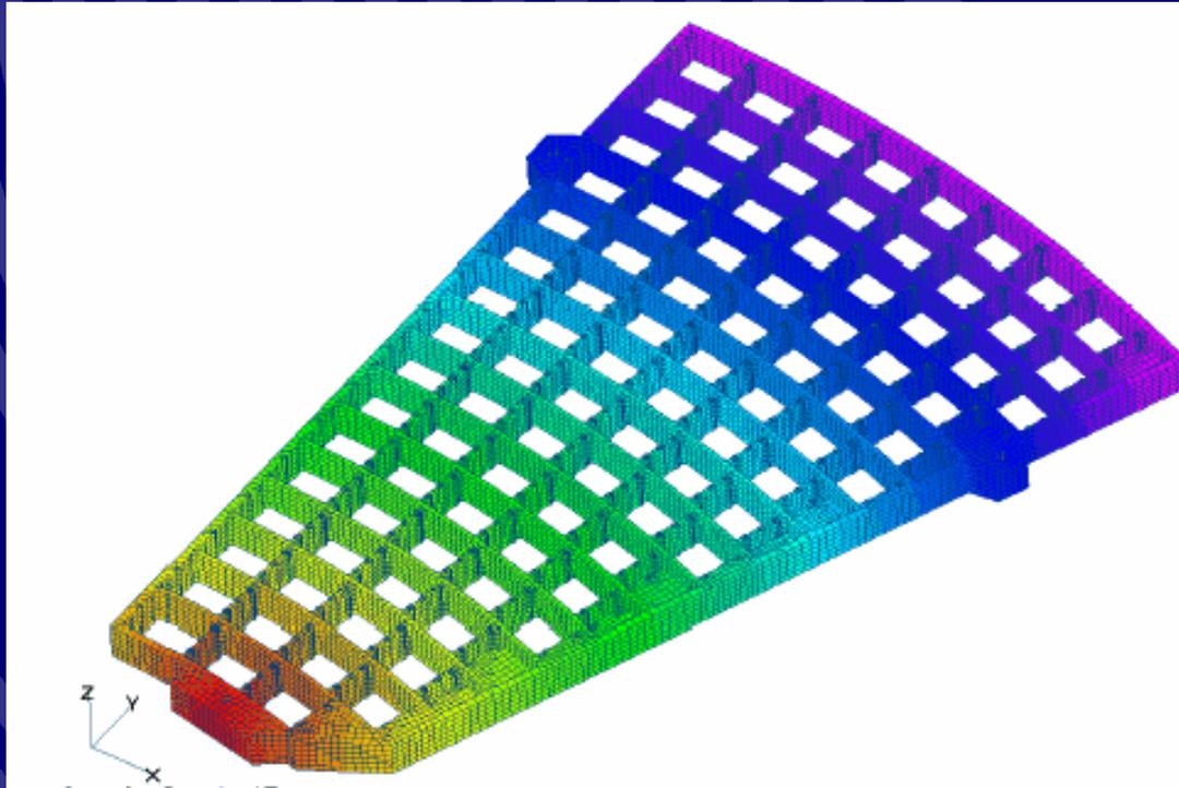
Finite Element Analysis by Keyser-Trede. Color shows temperature distribution across the petal. 3 attachment points/petal. 16 petals in total. Fixed alignment.
