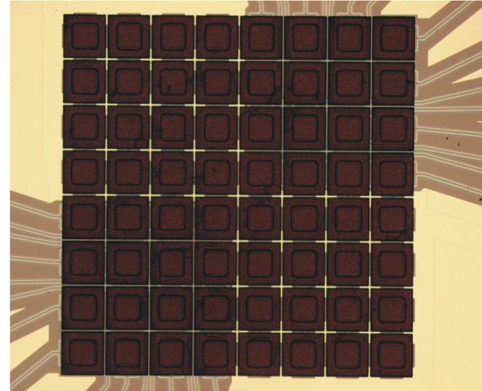
8x8 development TES array for Con-X with 250  $\mu\text{m}$  pixels
