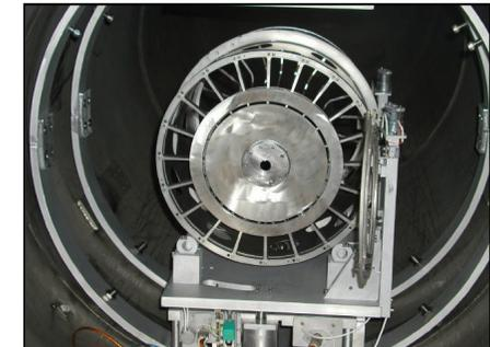
Single shell nickel mirror in X-ray test
