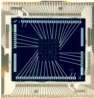
*Suzaku* X-ray calorimeter array achieved 7 eV resolution on orbit
