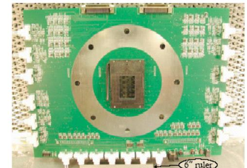
EDCCD: Large motherboard and camera plate (MIT)
