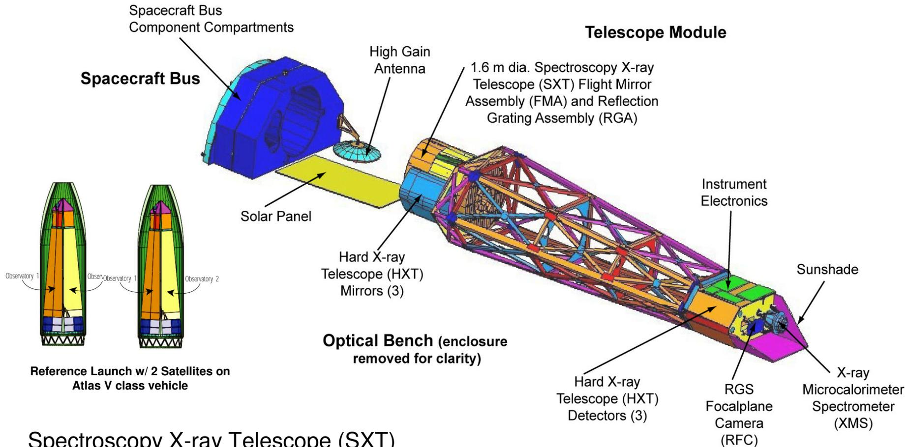
Spectroscopy X-ray Telescope (SXT)
