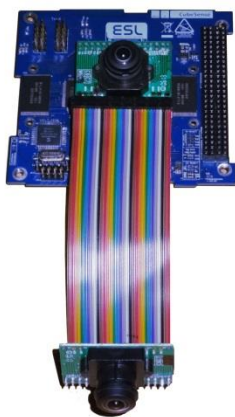
Figure 1 CubeSense sun and nadir sensor
